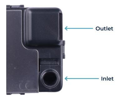
The sensor uses an active airflow to sample the particles. In order to maintain accuracy, we advise you to put the inlet directly to the air you want to monitor. If integration is difficult, you can add a duct made with antistatic materials and with an internal diameter of 8 to 9 mm. The maximum length of the duct must be 100 cm.
