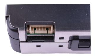
The connector is a 6 PIN one. You can use an ADAM TECH 125CH-B-06 reference to connect with or an equivalent, like a MOLEX 51021-0600.
