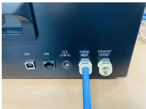
Purge Inlet - 1/8" Tube connect to Clean Air
