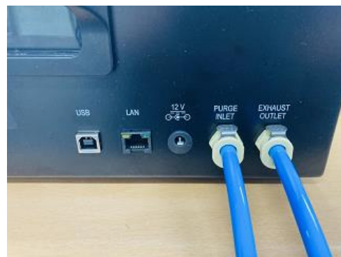
Exhaust Outlet - 1/8" Tube connect to ventilation
