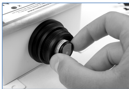
Figure 17 - Seating the MiniPID 2 back into the TVOC 2 sensor housing
