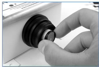
Figure 17 - Seating the MiniPID 2 back into the TVOC 2 sensor housing
