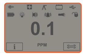
The main central viewing screen will display readings in large numbers only, up to 4 digits and decimal place will display 0.0 ppm to 5,000 ppm. When the maximum range is exceeded and the sensor over-ranges, the display will show '9999'. Two soft key areas have been set aside as soft key indicators. The area between the soft key indicators displays the measurement units.
