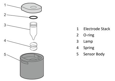
Discard the removed (old) Electrode Stack, carefully removing the Lamp if still attached.
