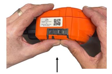
Once you hear it has engaged, push the rest of the sensor cover to the instrument body and screw the bottom left hand screw into place using the 3mm A/F allen key.
