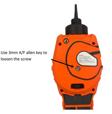
Once the screw is loose, gently pull the right side of the sensor cover from the instrument body until you feel that the sensor cover has unengaged from the inlet/outlet ports. Once it is unengaged, gently pull the entire sensor cover from the instrument body.
