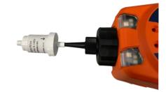
Press **Enter** to start the 'zero' countdown. At the end of the count down a tick ' $\checkmark$ ' will appear, indicating that the Zero has been accepted. Disconnect the Carbon Filter Assembly and replace the cap ends. The useful life of the Carbon Filter Assembly will be shortened if the Carbon Filter Assembly is open to atmosphere for prolonged periods.
