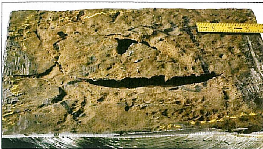
Figure 4 Cliffy notches and holes on the surface
